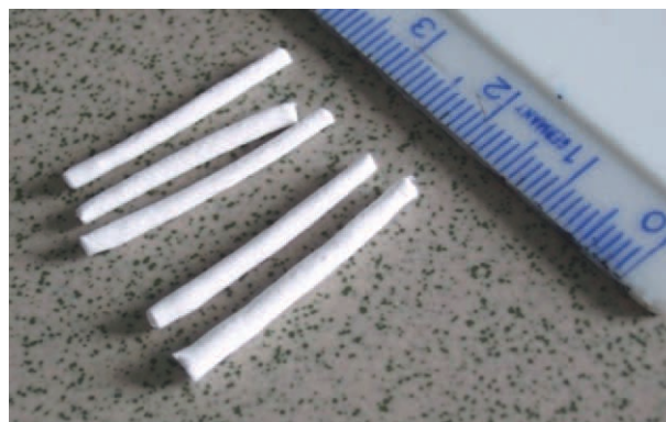
Figure 2. Photograph of manufactured nerve guidance channels. [Color figure can be viewed in the online issue, which is available at wileyonlinelibrary.com ]
